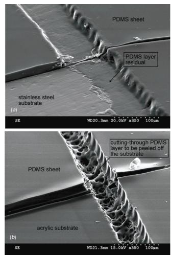
**Figure 3.** Cutting a 22  $\mu$ m PDMS sheet on substrates made of different materials. The PDMS layer on the bottom left was knife cut and removed. (*a*) On a stainless steel substrate, the PDMS layer cannot be cut through totally even with large laser power, leaving a thin layer of the PDMS residual on the substrate. (*b*) On an acrylic substrate, the laser can cut through the PDMS layer, leaving a groove over the acrylic surface.
