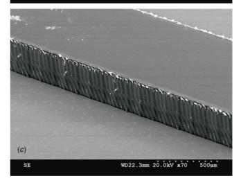
**Figure 6.** (*a*) At 1000 PPI, the sidewall is neat and clean when cutting the PDMS with a depth smaller than 200  $\mu$ m and a line width of above 60  $\mu$ m. (*b*) Debris appeared on the upper corner when cutting through a 300  $\mu$ m thick PDMS sheet at 1000 PPI. (*c*) When reducing the resolution to 600 PPI (~24 pulses per mm), the 300  $\mu$ m thick PDMS was cut through with little debris.
