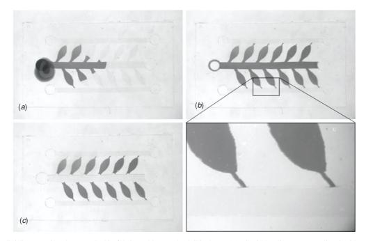
**Figure 7.** Microfluidic test using the PDMS chip fabricated by a pulsed  $CO_2$  laser. (*a*) Liquid loading process. (*b*) Liquid retained in the leaf reactors without leaking to the air venting channels due to confinement of the narrow openings of the passive valves. (*c*) Liquid remained inside the leaf reactors after removing the liquid in the stem channel by an absorbent.
