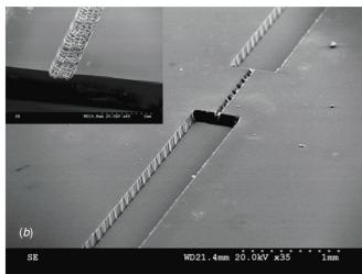
**Figure 5.** (*a*) Cross-sectional view of a PDMS microchannel with a height of 7  $\mu$ m which is controllable by forming a PDMS layer of the same thickness for laser through-cutting. (*b*) Channels with different widths and depths formed by a combined use of the through-cutting and the blind-engraving techniques. The wide channel has a smoother bottom when compared with the channel bottom formed by the raster scan (the inset).
