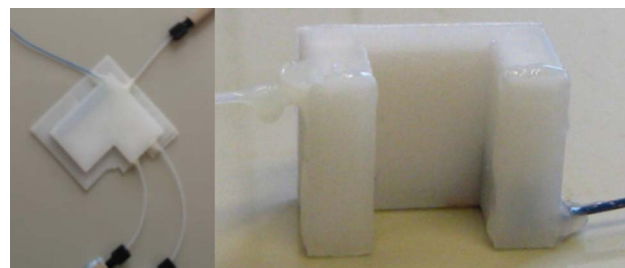
Fig. 6 Physical set-up of the 3D-printed reactionware used in the polyoxometalate syntheses. (Left) Three inlet device (R2) used with inlets of Na 2 MoO 4 ·2H 2 O, HCl (aq) and NH 2 NH 2 ·2HCl. (Right) One inlet device (R3) where HCl is flowed through silos containing solid Na 2 MoO 4 ·2H 2 O and hydrazine dihydrochloride, respectively.
