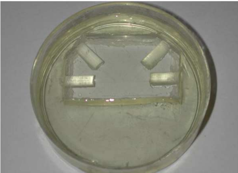
Fig. 5. The final epoxy mold.
