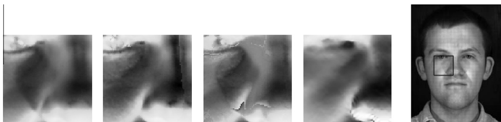
Fig. 8. Image of the vertical component of the surface normal (lighter areas indicate more downward pointing normals) for a region of a face in shadow. From left: estimates using standard four-source PS, using the proposed new algorithm, using the Solomon and Ikeuchi method, using the 3dMD scanner.
