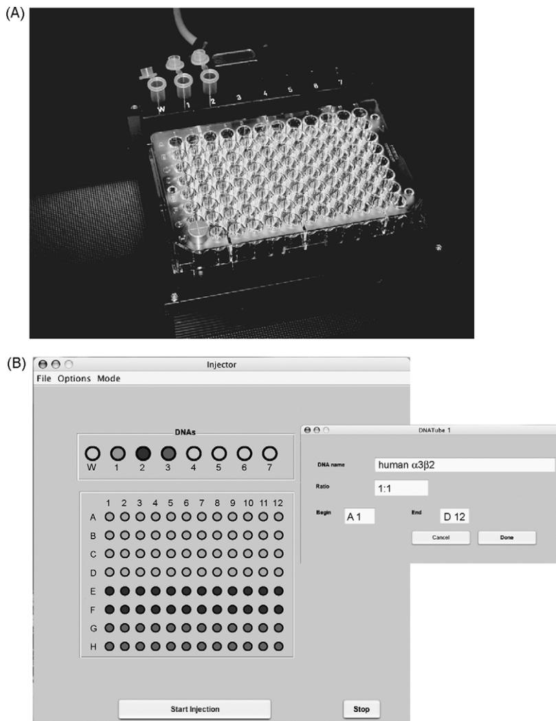
Fig. 4. (A) Illustration of the microplate carrier showing a 96-well microplate with the calibration guide and tube rack for the rinse solution and cDNAs. (B) Screen-capture of the window for entry of the cDNA information and selection of the wells to be injected.
