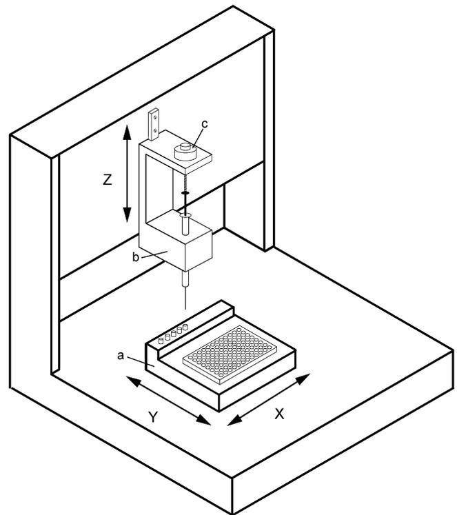
Fig. 2. Schematic illustration showing the main parts of the injection machine. The tube rack and microplate containing the cells to be injected are located on the microplate carrier, which floats on an air cushion and moves in the *X* and *Y* planes. The assembly (b) holds the microdispenser syringe and moves in the *Z* plane on a precision rail controlled by a linear actuator. A second linear actuator (c) controls the movement of the microdispenser piston.
