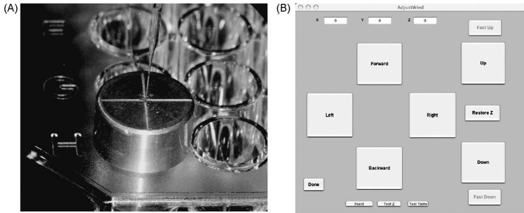
Fig. 3. Photograph of calibration guide and on-screen control pad for adjusting the reference position of injection pipette. The injection pipette is adjusted to the centre of the cross using the on-screen control pad.
