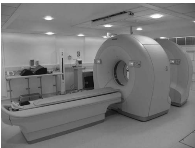
FIGURE 15.1 A GEMINI time-of-flight PET/CT. The PET/CT scanner consists of two devices; the first is a 64-slice CT and then the scanner table with the patient is moved to the second device, a time-of-flight PET.
