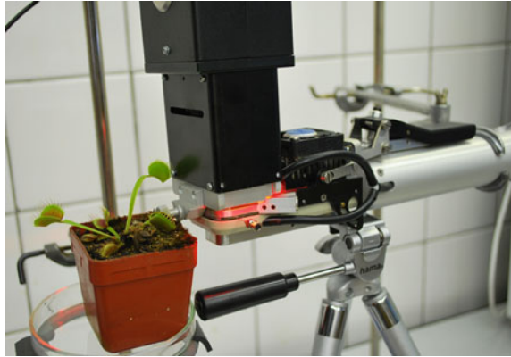
Fig. 2.1 Experimental setup. The trap of Venus flytrap ( D. muscipula ) is enclosed in hermetically closed gas exchange cuvette with attached fluorocamera. The thin wire in the needle from syringe is hermetically sealed and used for trigger hair stimulation
